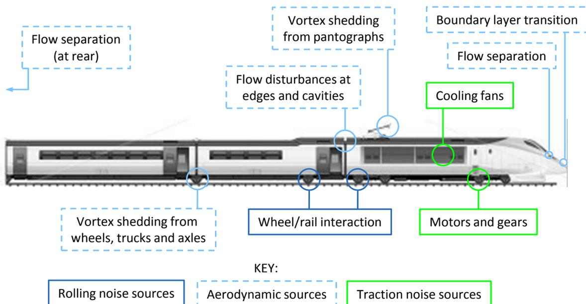
**Figure 1: Exterior noise sources on high-speed trains**
