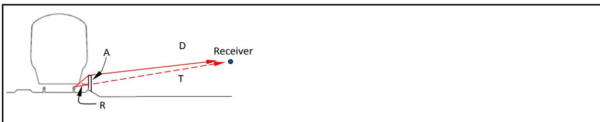
Noise barriers reduce noise levels at a receiver behind the barrier by obstructing the direct transmission of airborne sound emanating from the source in front of the barrier (in this case, noise generated at the wheel/rail interface). Sound waves are either reflected back from the barrier, absorbed by the barrier, transmitted through it, or are diffracted<sup>1</sup> over the top of the barrier (see Figure 2).
