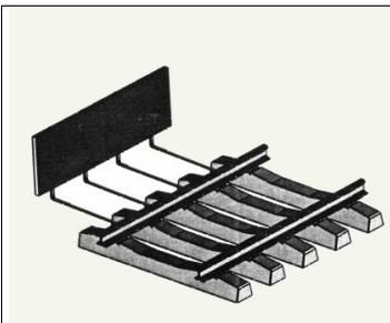
A further example of a low-height barrier is one where the barrier is fastened to the rail (Figure 5; it is unclear whether this is the actual rail or the sleepers) and, it is assumed, does therefore not require conventional foundations. No examples of this design in practical use have been identified and it is unclear whether the design has progressed beyond the concept stage.
