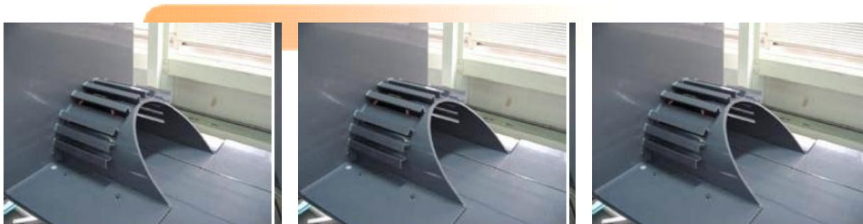
(a) Tunnel hood with 45° inclination and longitudinal slots
