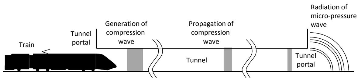
**Figure 2: The creation of micro-pressure waves resulting in noises at the exit of rail tunnels**
