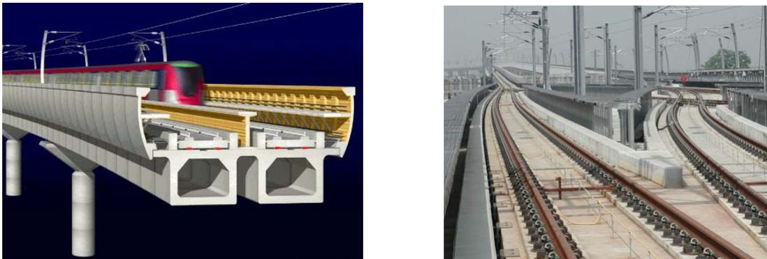
**Figure 3: Kowloon Canton Railway Corporation viaduct in Hong Kong with floating slab track, absorptive noise barrier and under-walkway absorptive plenum** (from Wilson, 2004)
